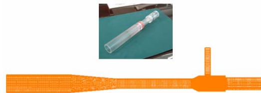
Fig. 3. The ejector model with trim cell mesh generation (inset: real ejector).
